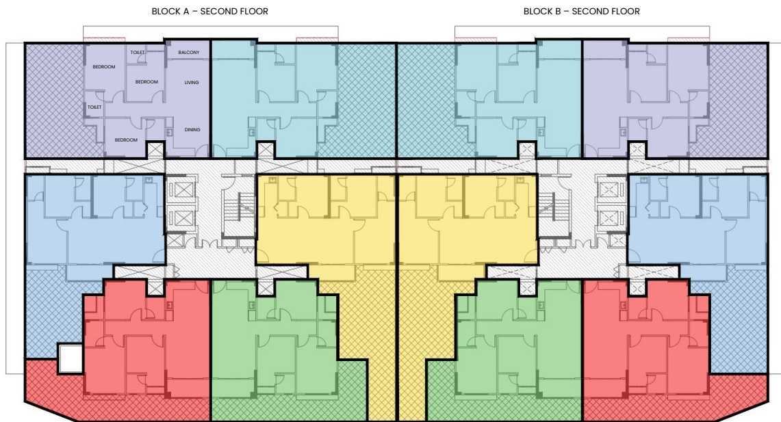
Figure 6: Typical Apartment types and Floor area with Terrace provision for Residential Apartments
